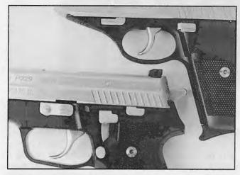
P230 (top) has both a hammer-drop lever and a disassembly lever in approximately the same location as those of the P229 (bottom). P230 has no slide-stop lever and the magazine catch/release has been moved to the heel of the grip-frame in back of the magazine-well.
